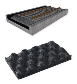
The RailMat **Ballast Mat Damper** is a vibration damper made of recycled rubber that is installed under the ballast of a railroad. It reduces vibrations of ballasted tracks in urban areas (up to -20 dB @ 63 Hz).
