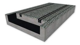
The **Slab Mat Damper** is a resilient mat made of natural recycled rubber that surrounds floating slabs of concrete railway tracks and significantly reduces the level of vibration in urban areas (-20 dB @ 63Hz).
